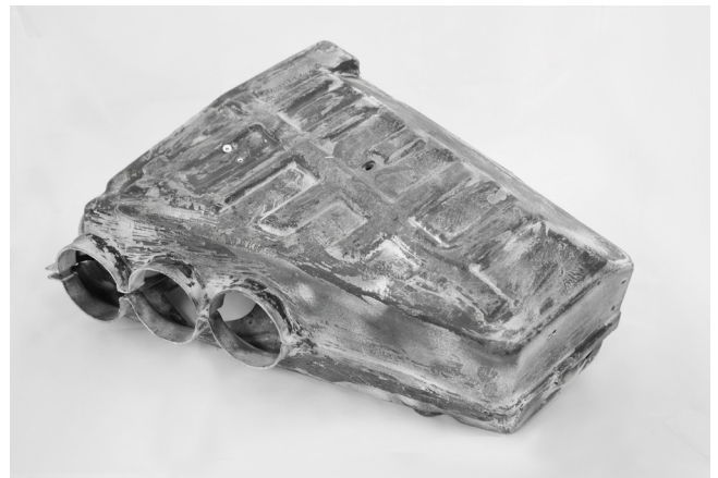
Obsolete air conditioning duct for historic supercar that needed replacing.
